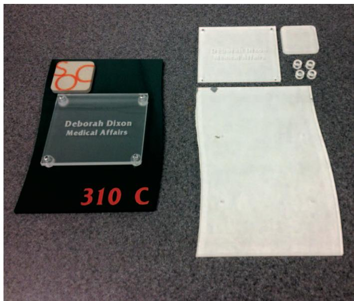
You can see that we cut all the components for this rather complex door sign on the laser from a single piece of acrylic—even the standoffs.
